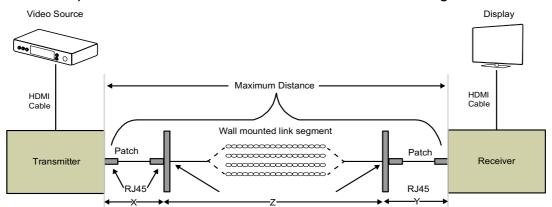
The lengths of the cables used in three segments shall follow the specification below:
