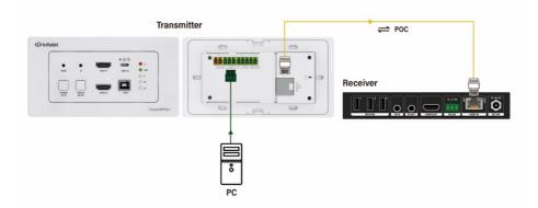
2) If the far-end third-party device (e.g. projector) need be controlled by PC, please connect the third party device (e.g. projector) to the RS232 port of receiver. The connection diagram shown as below:
