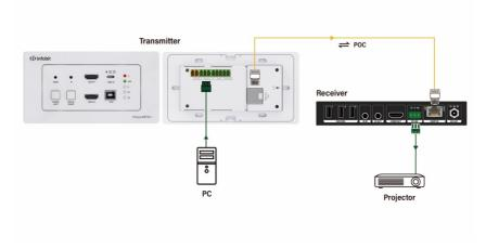
3) If the switcher needs to be controlled by receiver end, the control device (e.g. PC) can be connected to the RS232 port of the receiver, the connection diagram shown as below:
