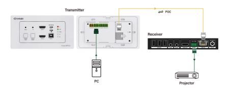
3) If the switcher needs to be controlled by receiver end, the control device (e.g. PC) can be connected to the RS232 port of the receiver, the connection diagram shown as below:
