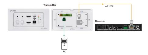
2) If the far-end third-party device (e.g. projector) need be controlled by PC, please connect the third party device (e.g. projector) to the RS232 port of receiver. The connection diagram shown as below:
