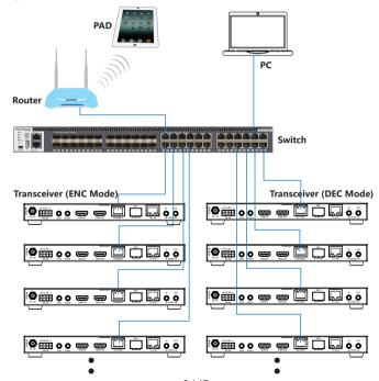
**Step 2:** Set the PC's IP address to the same network segment with Switch, for instance, set the IP address to be 169.254.3.30 and Subnet mask to be 255.255.0.0.
