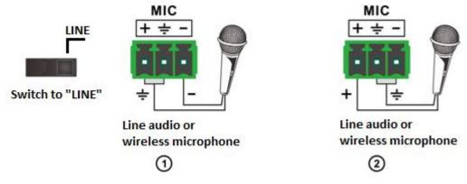
2) Balanced connection: "+" connects to positive, "-" connects to negative and "= "connects to ground.
