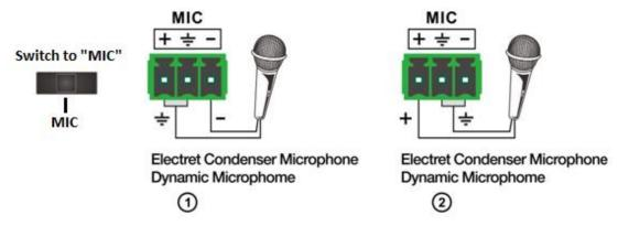
2) Balanced connection: "+" connects to positive, "-" connects to negative and "= "connects to ground.
