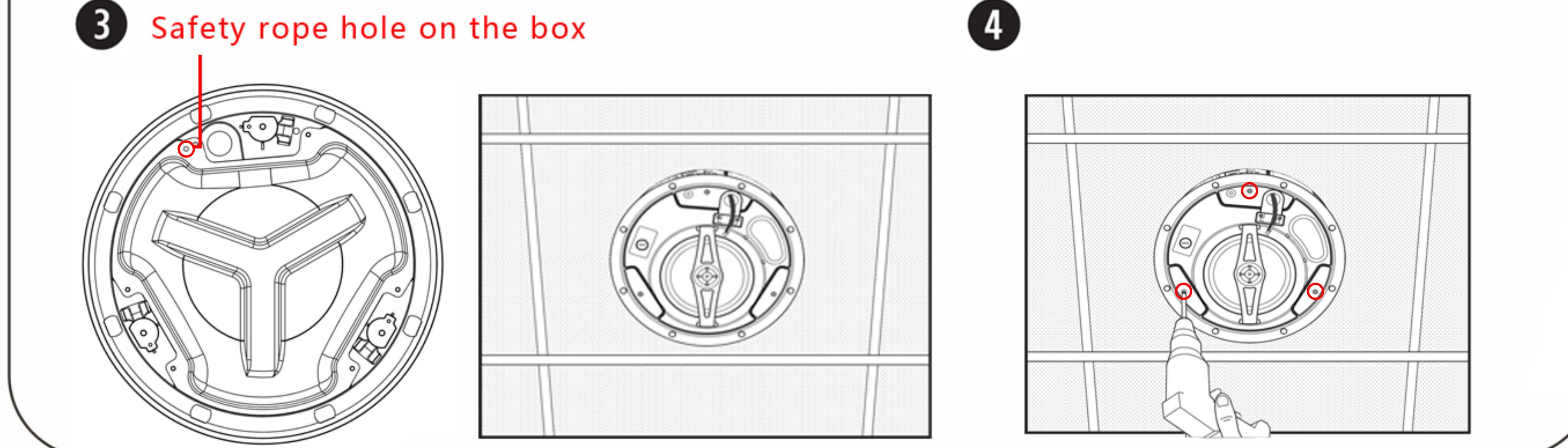
5. Connect the terminal to the speaker cable. Tie one end of the grille mounting rope into one of the four safety rope holes on the back of the grille. Tie the other end of the grille safety cable to the cable pin and insert it into the cable pin hole on the speaker.
