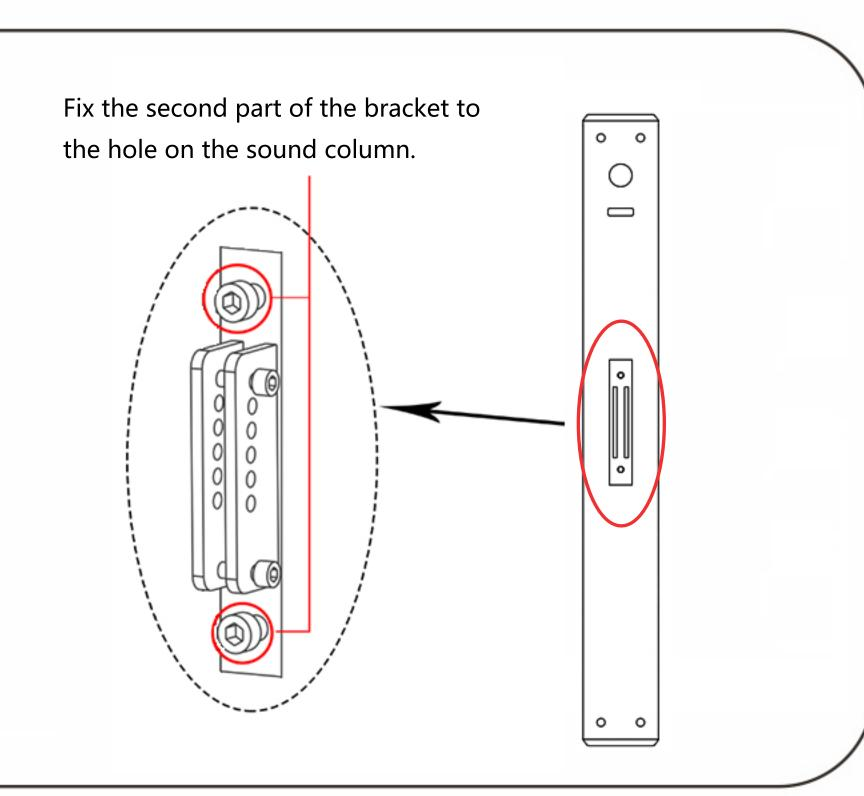
5. First put the assembled bracket under the second Hook the screws to the hook grooves on the first bracket, then align the angle adjustment holes above the two brackets according to the required angle, lock the screws, and the assembly is completed.
