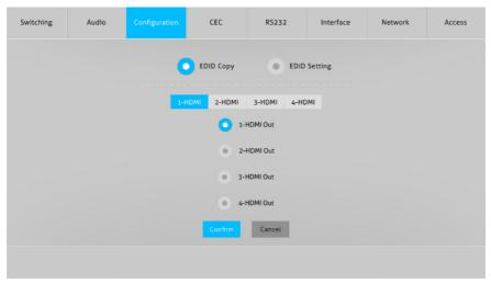
• Copy the EDID of the selected output device to one or more input source device.
