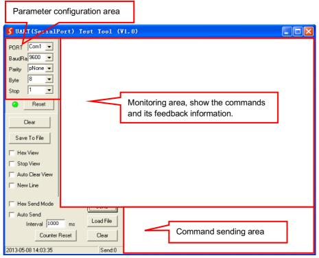
Set the parameters (baud rate, data bit, stop bit and parity bit) correctly to ensure reliable RS232 control.
