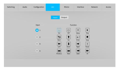
Select one input source device to be controlled, and then press function buttons.
