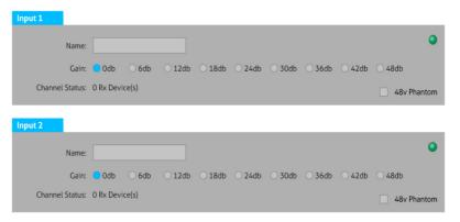
**Name:** Reports the Dante transmitter channel name for corresponding analog input and rename the input.
