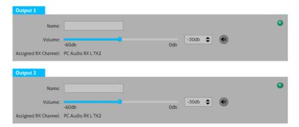
**Name:** Reports the Dante receiver channel name for corresponding analog output and rename the output.
