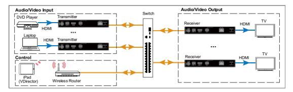
Configure the wireless router properly, and then connect your phone/tablet to the Wi-Fi network. Then launch VDirector, VDirector starts searching for online devices, and the following main screen appears:
