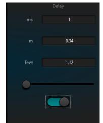
**ms:** sets the delay time of the delay er. This value ranged from 1 to 1,200 ms.meters and feet are converted unit values of milliseconds.
