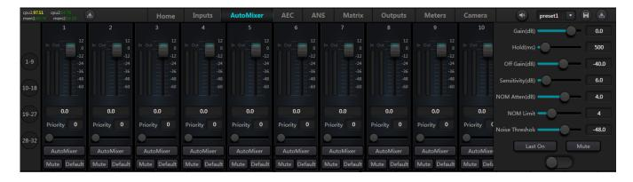
The threshold automatic mixer is based on the noise gate development, each channel has a noise gate, which is either open or closed.
