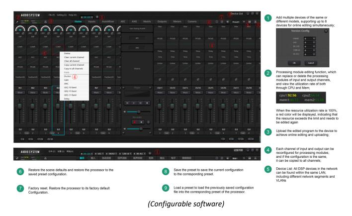
At the same time, we also support functions such as online editing for up to 8 devices, saving configurations to devices (uploading to devices), restoring presets, restoring factory settings, saving presets, and loading presets.
