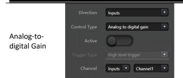
Analog-to-digital gain is very useful when connecting potentiometer externally. It may adjust input or output channel gain. It looks like rotary encoder. The difference between them is potentiometer analogs and adjusts voltage and current while encoder is digital and transmit the binary codes of 0 and 1.
