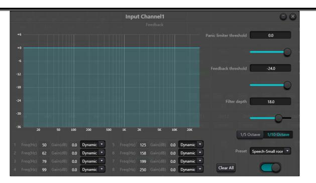
The feedback inhibition module has the following adjustable parameters:
