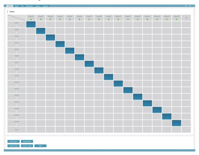
The Matrix Switching page displays the names and statuses of all input and output ports. The green light under the name of the input/output port indicates that there are connected signal sources or display devices; The gray light indicates that no signal sources or display devices are connected.
