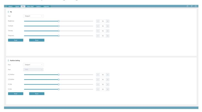
Only the output port supports picture quality adjustment. The value ranges from 0 to 32, and all values after resetting are 16.
