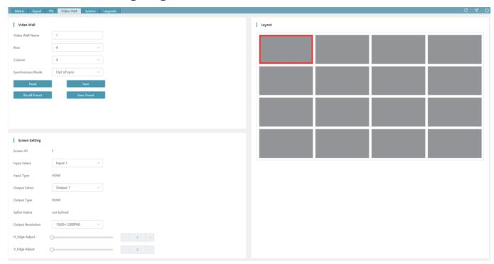
The number of rows and columns of the video wall ranges from 1 to 16. After the video wall is created, parts with more than 64 screens will not be displayed.
