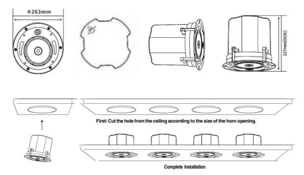
After the hole is completed, install the speaker in the direction of the figure and fix it.
