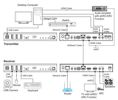
Note: Please press the eARC buttons on the front panel of the transmitter and receiver to enable the eARC/ARC function before operating the system.
