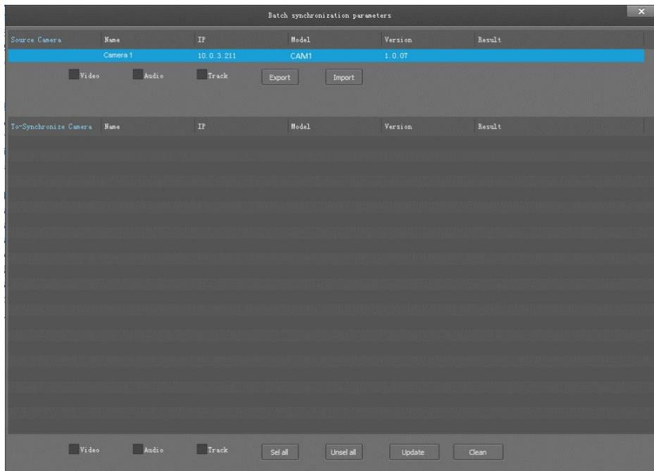
Select the camera to be synchronized of the same model which are currently managed and unselected, and then click any option or multiple options among the video, audio and track. After clicking the "Update", the current camera to be synchronized will be synchronized with the Source camera parameters.
