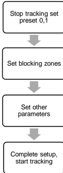
**Preset 0** and **Preset 1** are set as presets of full view generally, or as presets of any zoom or location. When there is no target, preset 0 or preset 1 could be chosen to have camera move to. Please refer to Basic Setting.
