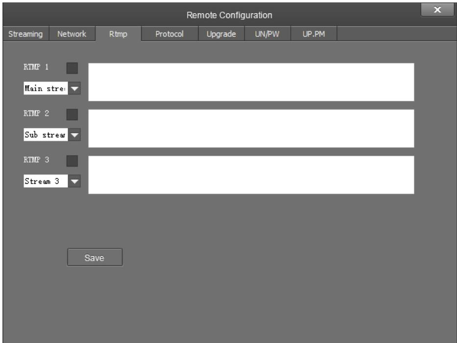
In RTMP1 and RTMP2, main stream, sub stream and third stream can be chosen to stream. Support common RTMP servers, such as red5, nginx, crtmpserver, fms, wowza.
