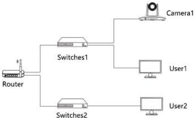
Please refer to the above diagram, user1 and user 2 are in the same router, they are considered as in the same LAN, connect the camera to the same LAN as where the PC is, and refer to below instructions as how to use the application software, then the camera can be found and connected
