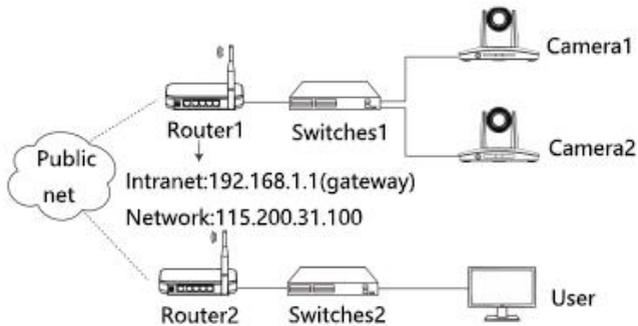
Please refer to the above diagram, user PC and the camera are in different routers, they are considered as in a WAN, in this condition, Client can't search and find the camera automatically. Client can still access the camera once below three conditions are satisfied.
