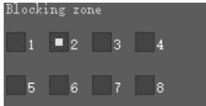
**Blocking zones:** To avoid incorrectly framing moving objects on screens, these 8 blocking zones are used to block screens in the full-view camera image, they can be configured independently, moving objects inside the blocking zones of the full-view camera will not be detected or framed.
