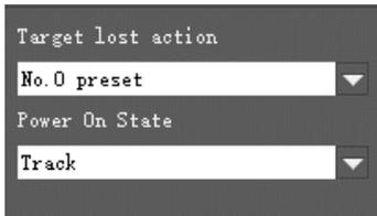
**Target Lost Action:** used to define the action to be performed if the camera loses the tracked object for a period of time.
