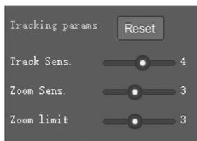
**Track Sens:** set sensitivity of tracking based on range of movement, if value is big, camera tracks at minor movement range.
