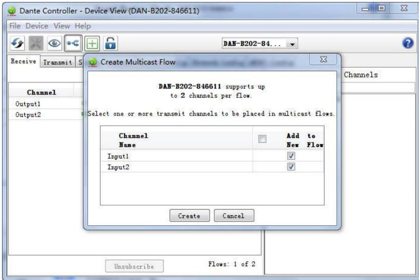
Click Transmit and delete the transmit flows for disabling multicast mode as the below:
