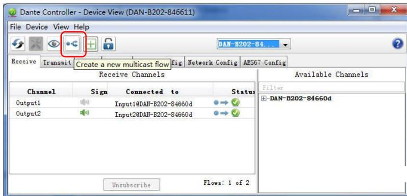
Select the device and tick the input channels.
