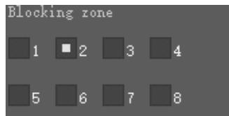
**Blocking zones:** there are 8 blocking zones shown in green rectangle, they can be configured independently. The moving objects inside the blocking zones of the full-view camera will not be detected and tracked while the tracking camera still tracks the lecturer.
