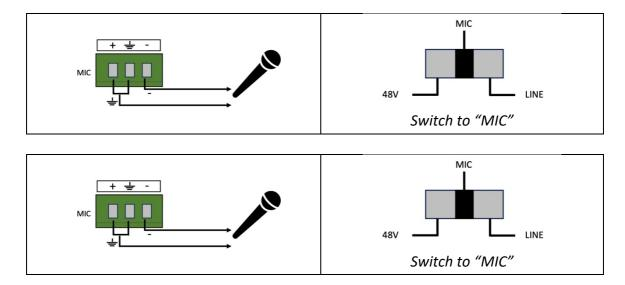
2) Balanced connection: "+" connects to positive, "-" connects to negative and "\( \blue{-}'' \) connects to ground.
