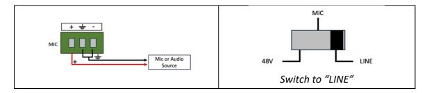
2) Balanced connection: "+" connects to positive, "-" connects to negative and "\( \blue{\subset} \)" connects to ground.
