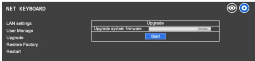
The upgrade function is used as the maintenance and update keyboard function. After entering the upgrade page, select the correct upgrade file, click "Start", and the device will restart automatically after the upgrade.
