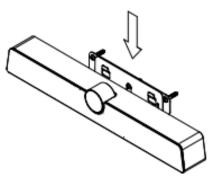
3. Use with panel: Fix the bracket onto the supporting bracket with screws, then place the integrated video conference terminal onto the bracket. (The bracket needs to be purchased separately.)
