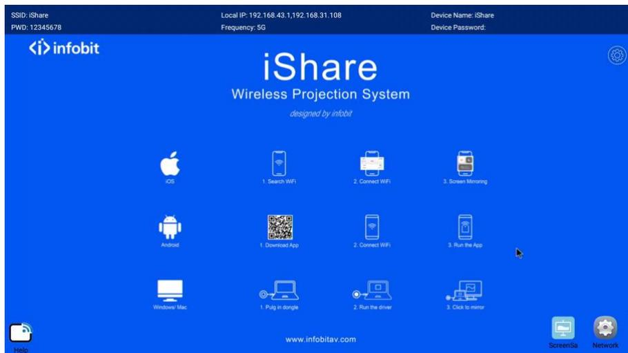
4. A USB mouse is required to set up iShare by plugging into receiver through USB port. Left click represents "Confirm" and right click represents "Back".
