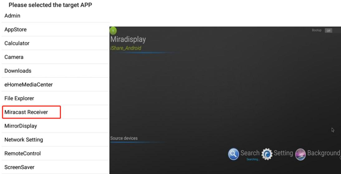
When your devices start to cast, sources devices will list the device model. If enable <Bootup>, the page will pop out automatically.
