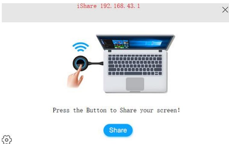
If the computer works with dongle for the first time, you have to run USBDisplay driver when it pops up after plugging in dongle, or follow My Computer->CD Drive USBDisplay to run the driver.
